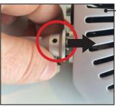
5. Slide the aluminum collar back over the connector so it is firmly pressed against the back of the laser as far as it can go and the large thumb screw is on the bottom as shown below. Ensure that the black plastic switch is being fully pressed by the aluminum collar as shown.
