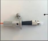
Loosen the adjustment set screw on the aluminum collar and slide the collar backwards to expose the connector.
