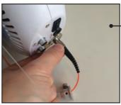
4. Remove the protective dust cap and screw the fiber to fiber port on the back of the laser. Take care not to touch the fiber tip.
